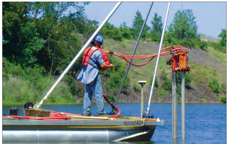
Above: Alpine Model M pneumatic mini-vibracore in operation
