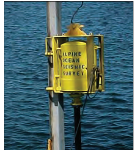
Below: Alpine Model E electric vibracore head
